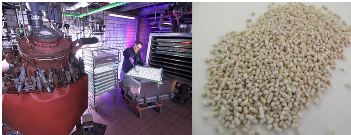
Figure 1: Photography of the 650L vessel for the demonstration of UiO-66 manufacture (left), photography of UiO-66 extrudates of 1mm in diameter for ammonia air purification filters 9 .
