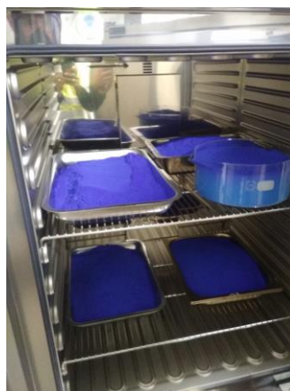
Figure 1: MOFs (HKUST-1) beads of 80 \mu\text{m} in diameter prepared by spray-drying process.
